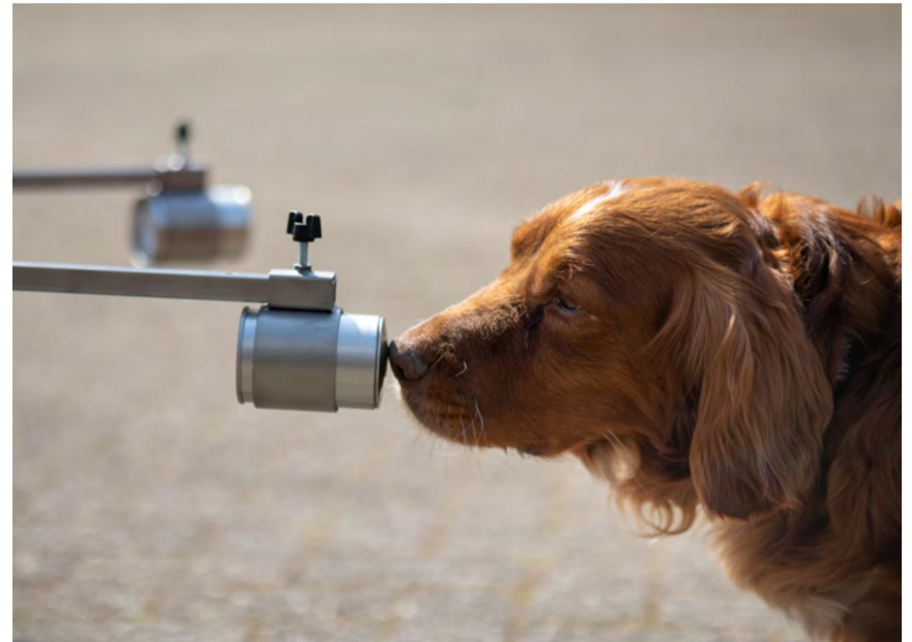
As soon as the dog puts his nose in a target, the sensor will log it and send it to the computer.
